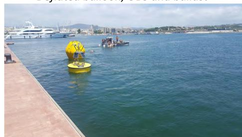
Bloated balloon, connected to buoys-OBS and ballast
